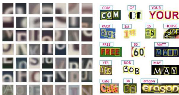
Fig. 9 Strokelets for scene text recognition [7]. In contrast to [32], the parts of characters (i.e. strokelets) are automatically learned from training data.
